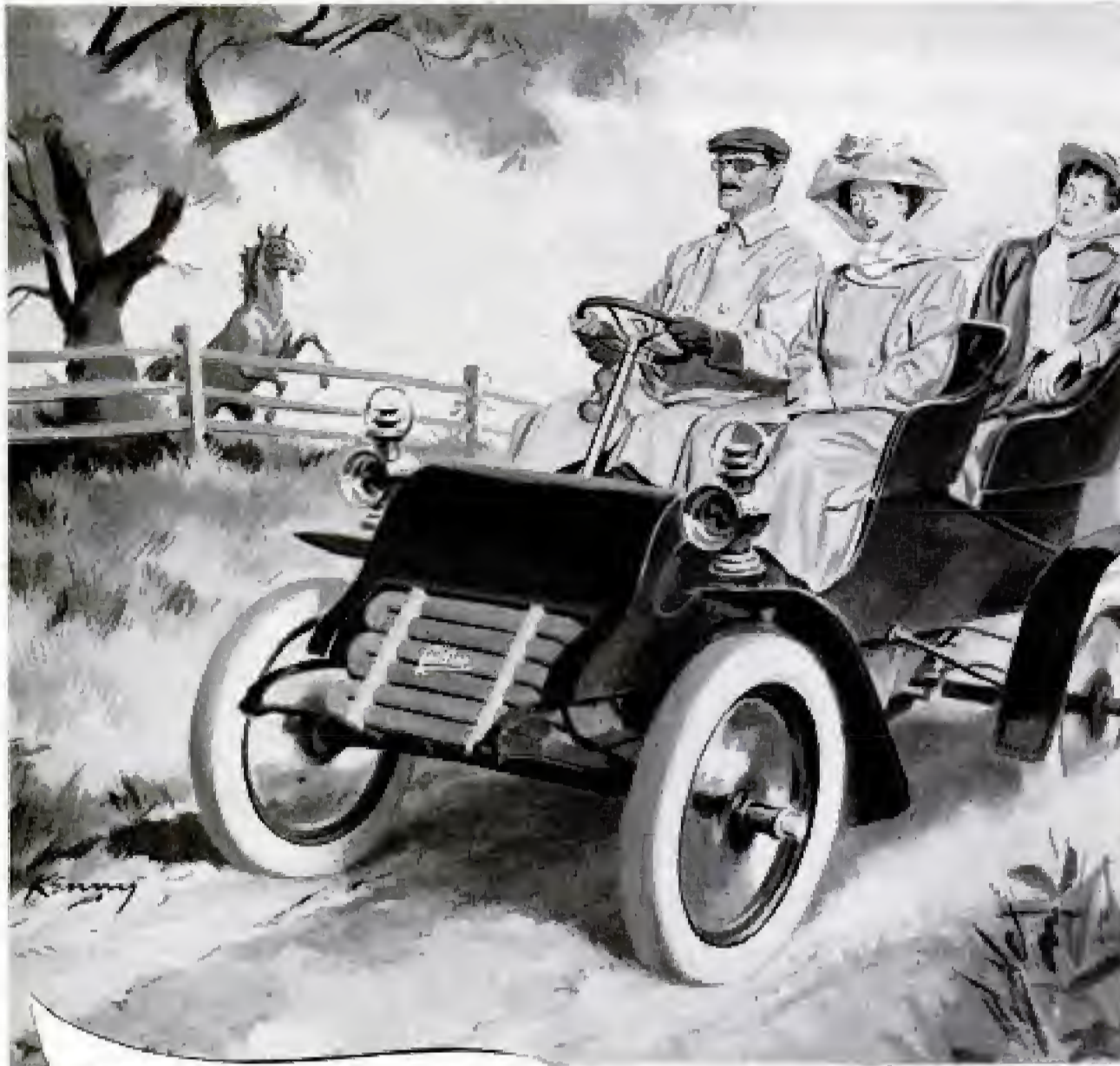
1902 CADILLAC featured a single-cylinder six and one-half horsepower engine under the seat. About 1700 of these Cadillacs were sold for around $750 each.
